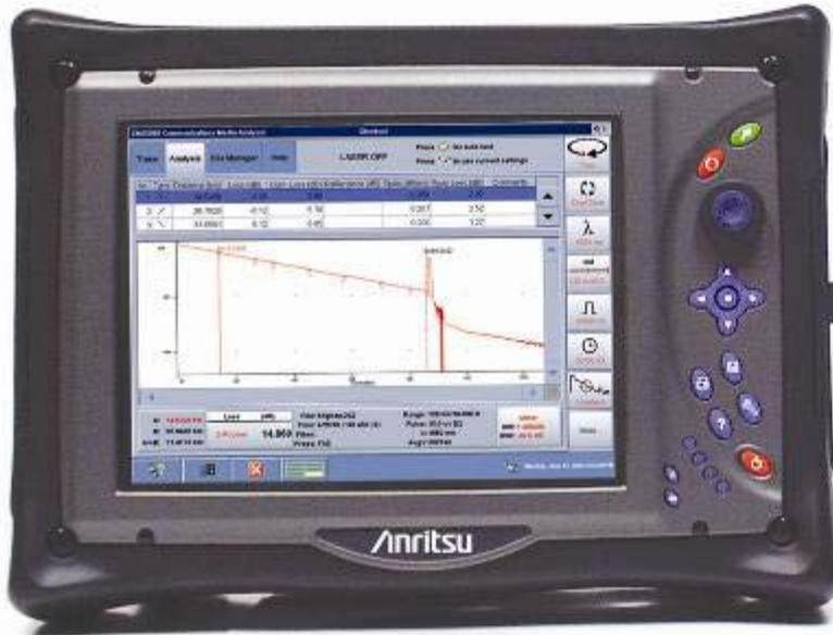
The compact size of the OTDR Application module allows another module (OTDR or test fiber box) to be inserted into a small bay adapter and up to three more into a medium or large bay adapter.
