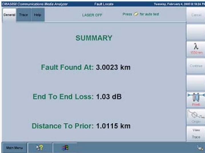
Fig.1: Fault Locate Mode - ease to read results
